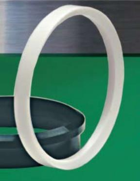
This connection is not over-engineered and requires very little maintenance or meticulous and time-consuming measurement upon installation, is easily repaired or replaced and is highly affordable. The wedge-shaped glass-filled PTFE ring compresses between two sturdy molded flanges across the connection to insure against corrosion of exposed box or collar steel surfaces.
